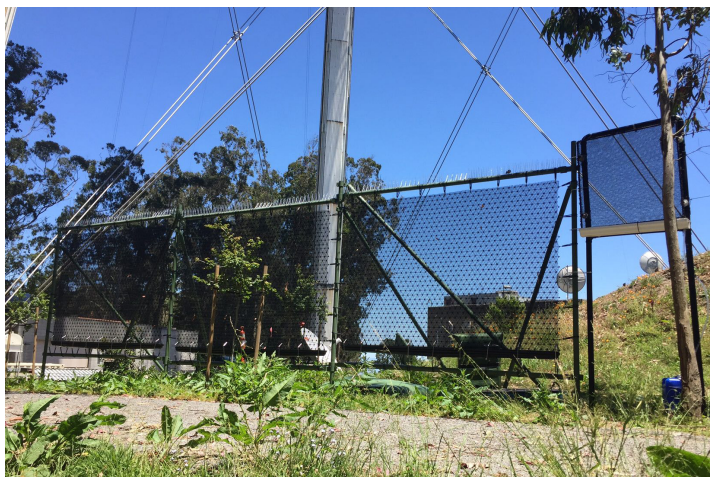
The German Water Foundation's CloudFisher fog collector and a new FogQuest fog catcher have different meshes
